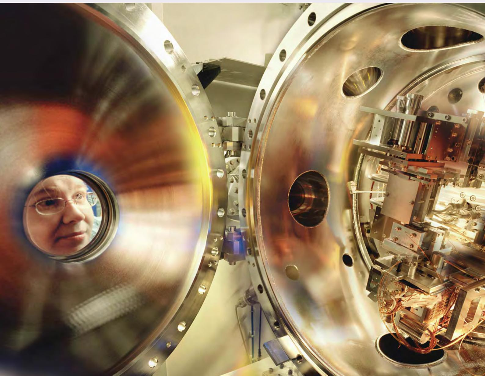
ESRF beamline for X-ray microscopy
